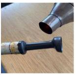
To minimize this affect, shrink the tube onto the larger dimension and allow to cool before returning to shrink the tube on to the smaller dimension.
