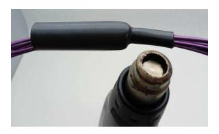
c. The heat should be applied in a controlled way by directing the air flow onto the tube for the whole length of the tube. This can be achieved by either rotating the assembly or the heat gun. See figure 2.
