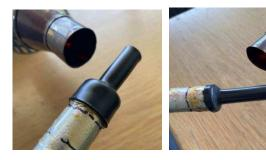
To minimize this affect, shrink the tube onto the larger dimension and allow to cool before returning to shrink the tube on to the smaller dimension.
