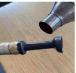
To minimize this affect, shrink the tube onto the larger dimension and allow to cool before returning to shrink the tube on to the smaller dimension.
