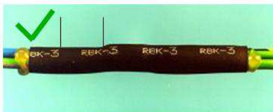
5. Tubing off centre (verify sealing)
