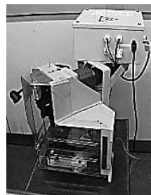
AMP 3K/40 Terminating Machine MOD CE 2161400-[] and AMP 5K/40 AMP Terminating Machines MOD CE 2151500-[]
