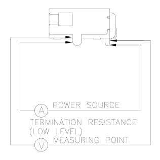
(1-2129458-1/-2 measuring point of Ground Shell & Ground Contact)
