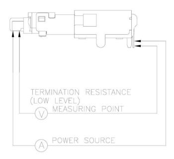
(1-2129458-1/-2 measuring point of Detect contact)
