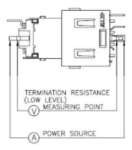
(2129567-1 measuring point of Detect contact)
