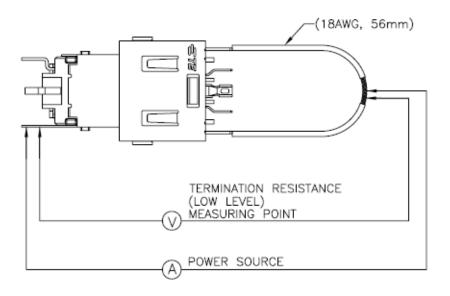
(2129567-1 measuring point of Ground contact)
