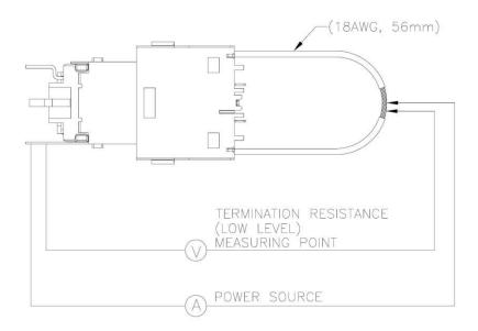
(1-2129458-1/-2 measuring point of Ground contact)
