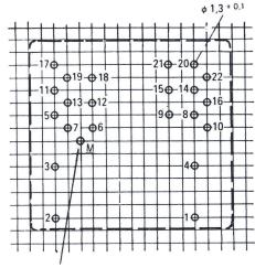
Hole M required only for relays with earth connection.
