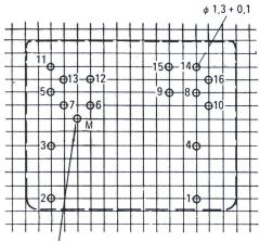
Hole M required only for relays with earth connection.
