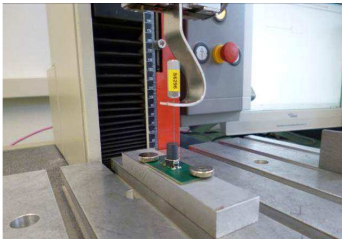
Fig. 7 Test Group AP: Test setup for gauge retention force
