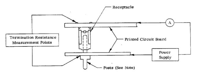
Note: Post plating shall be identical to receptacle plating when conducting tests, see Figure 5.
