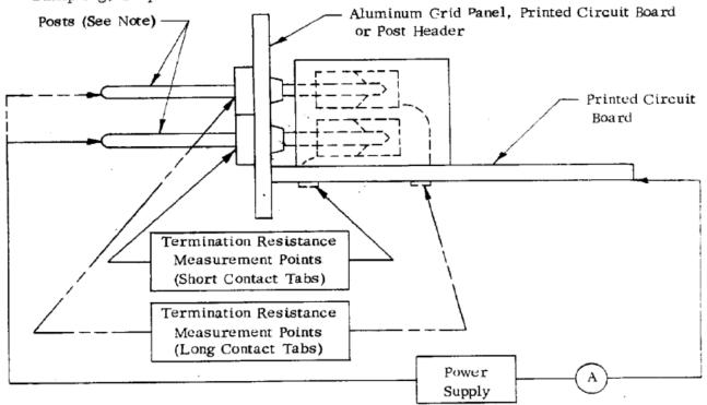
Note: Post plating shall be identical to receptacle plating when conducting tests, see Figure 5.
