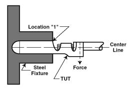
Fig. 1 Terminal Bend Resistance
