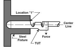
Fig. 1 Terminal Bend Resistance
