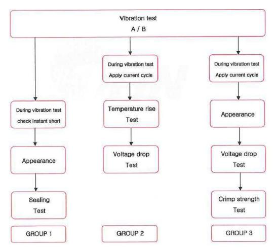
In the multipolar connector, Evaluation test at the same time for group 2/3
