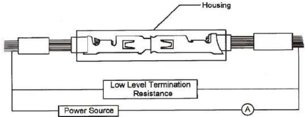
**NOTE** Bulk wire resistance shall be subtracted from resistance readings.
