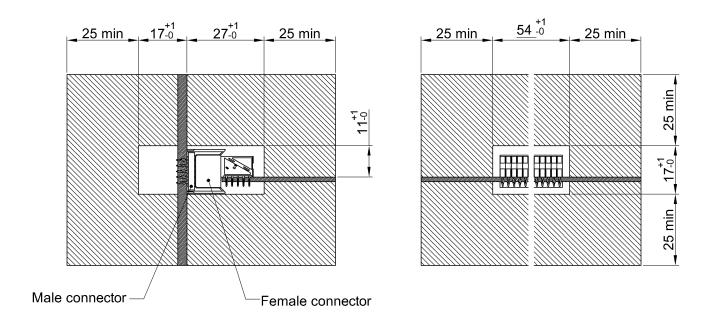
Figure 3: Fixture for dynamic stress tests.
