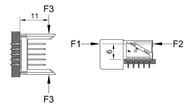
Figure 5: Test arrangement and application forces for static load test.
