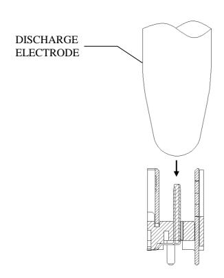
Fig.2 Test method of Electrostatic Discharge
