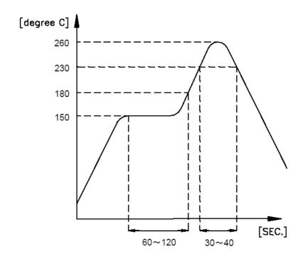
Fig.3 Temperature Profile of Reflow Soldering
