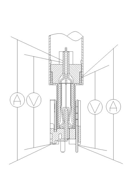
Fig.1 Contact and Shell Resistance Measuring point
