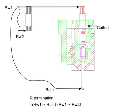
Low Level Contact Resistance Measurement Points Figure 3
