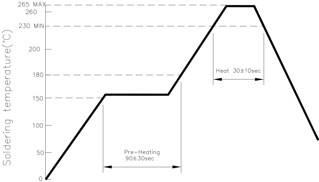
Fig.3 Temperature Profile of Reflow Soldering
