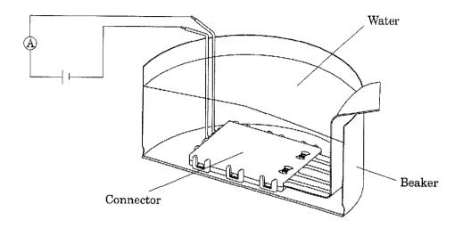
\*Immerse the connector in beaker filled with water
