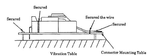
Fig. 9 Connector Mounting Methods of Low Frequency Vibration and Physical Shock Tests
