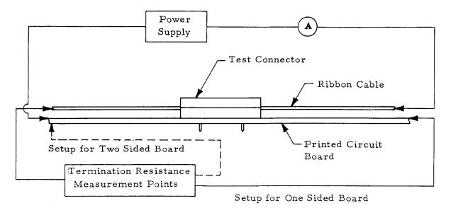
Figure 3 Termination Resistance Measurement Points
