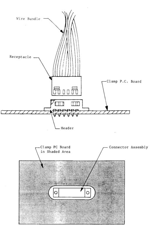
Figure 7 Mounting and Clamping Location for Vibration and Physical Shock
