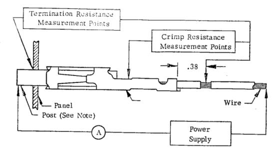
Note: Post plating shall be identical to receptacle plating when conducting tests, see Figure 4.
