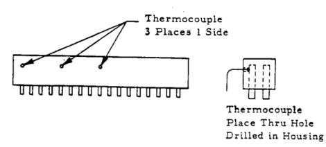
Figure 5 Resistance and Temperature Measurement Points
