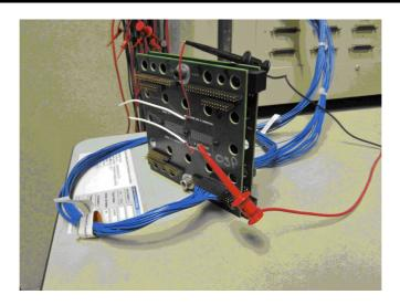
Figure 3 LLCR Measurement Points
