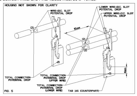
5.3.2 Current Cycling (DIN EN60998-2-3 was Spec.#109-51) at max. operating temperature (115°C as per para. 3.4.2)
