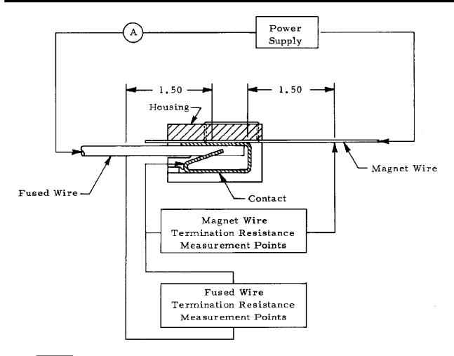
Termination resistance equals millivolts divided by test current less resistance of 1.5 inches of wire.
