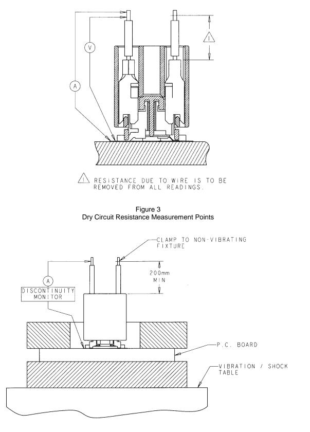
Figure 4 Vibration & Mechanical Shock Mounting Fixture
