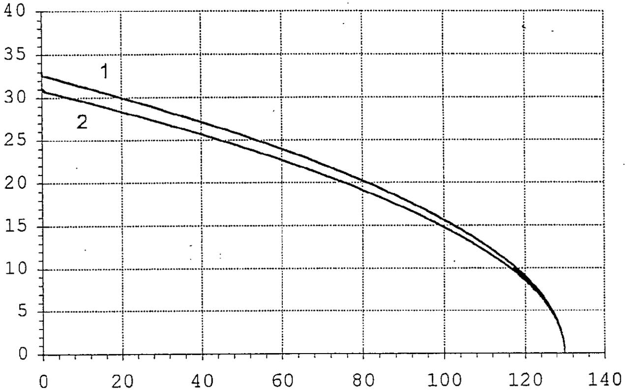
Diagram 3e: current carrying capacity in housing
