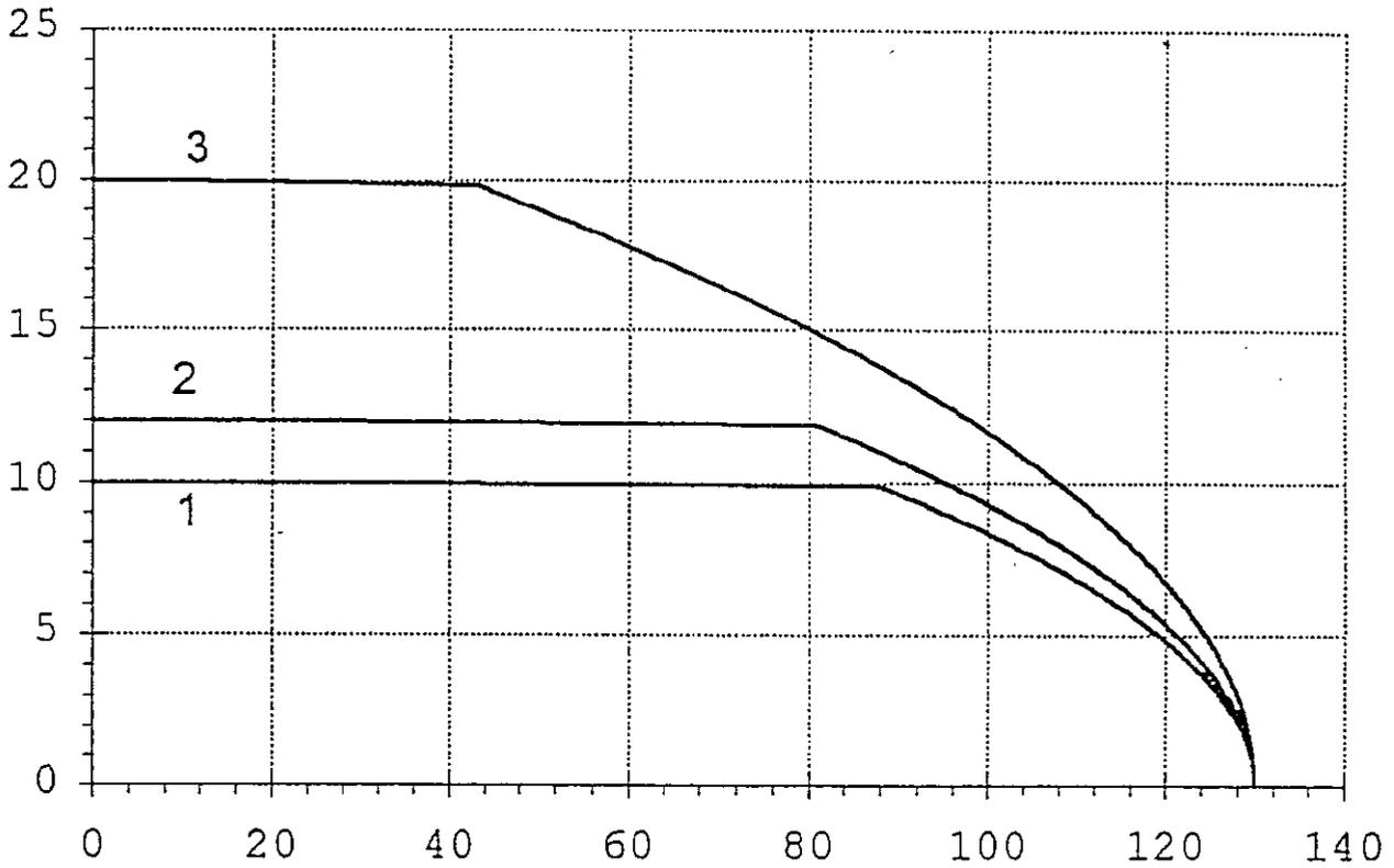
Diagram 2a : current carrying capacity „free in air“
