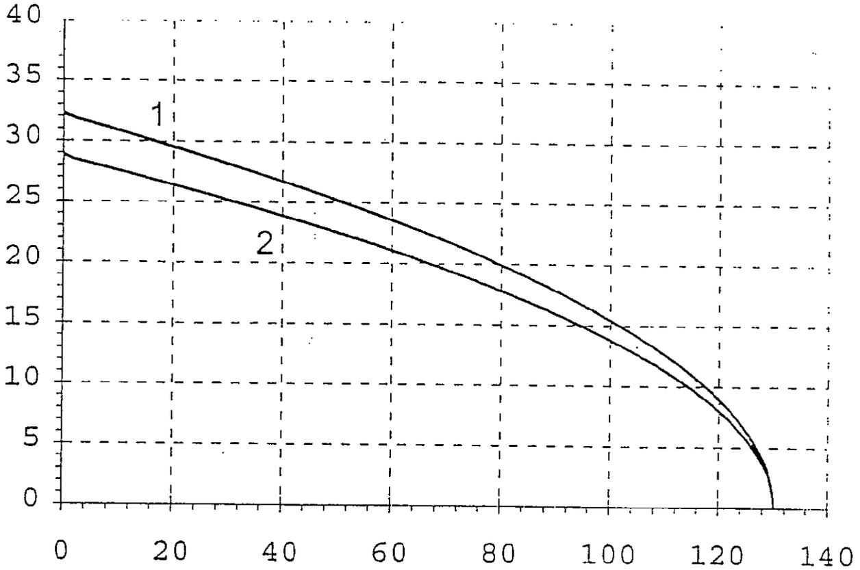
Diagram 4d : current carrying capacity (before and after stress test)
