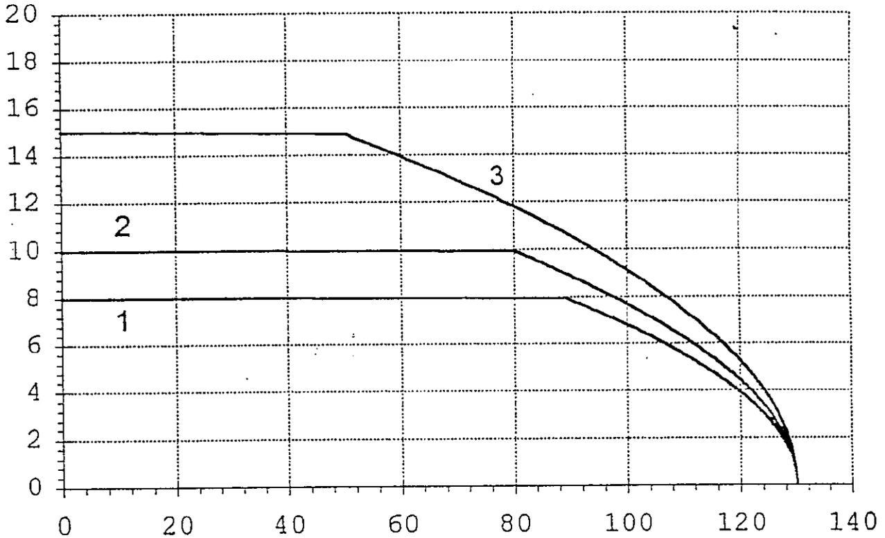
Diagram 3a : current carrying capacity in housing
