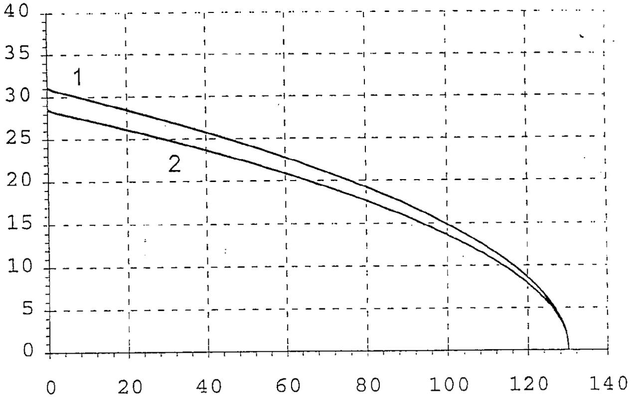
Diagram 4b : current carrying capacity (before and after electrical stress test)
