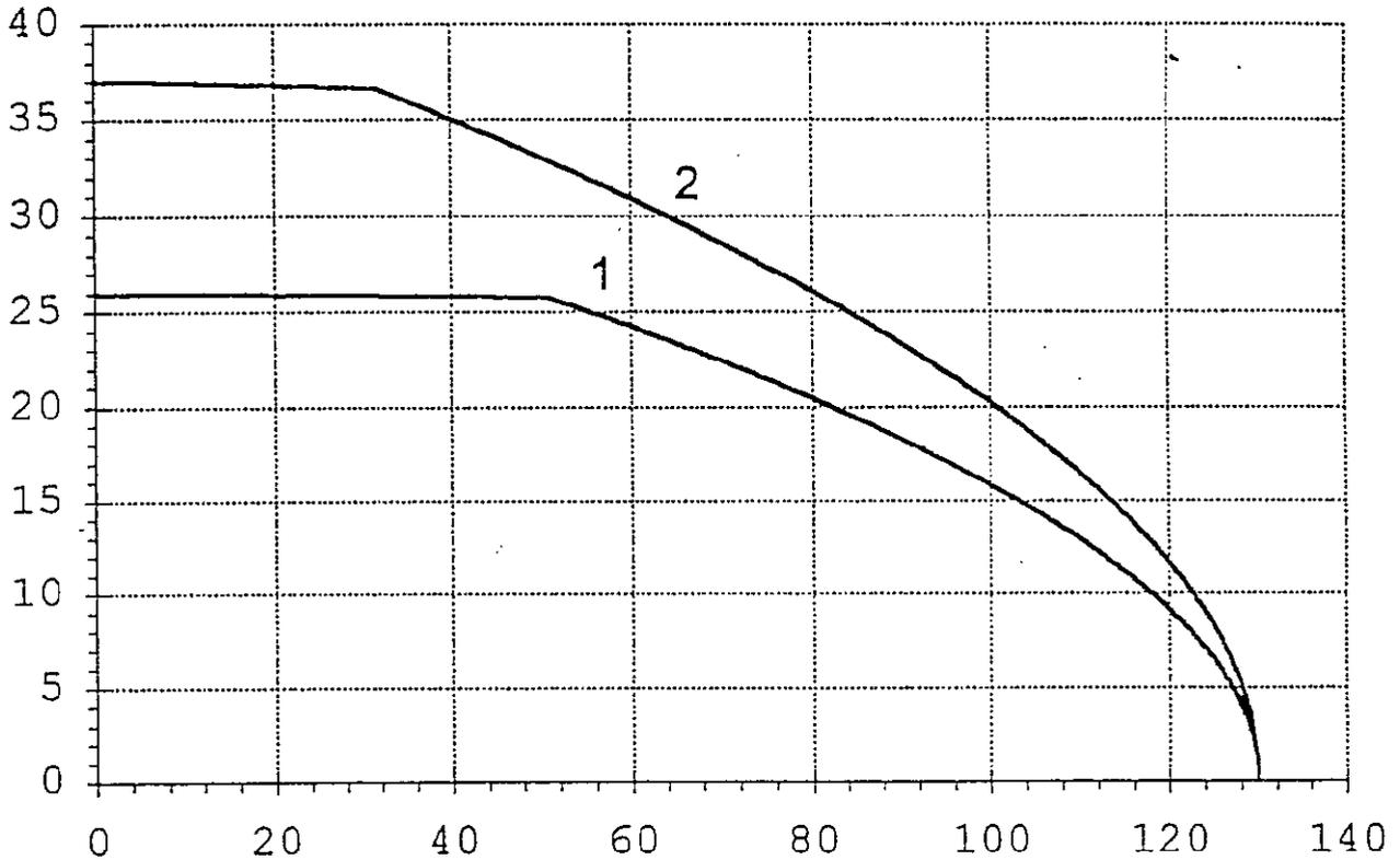
Diagram 3d : current carrying capacity in housing
