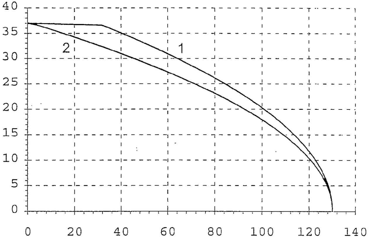
Diagram 4c : current carrying capacity (before and after electrical stress test)
