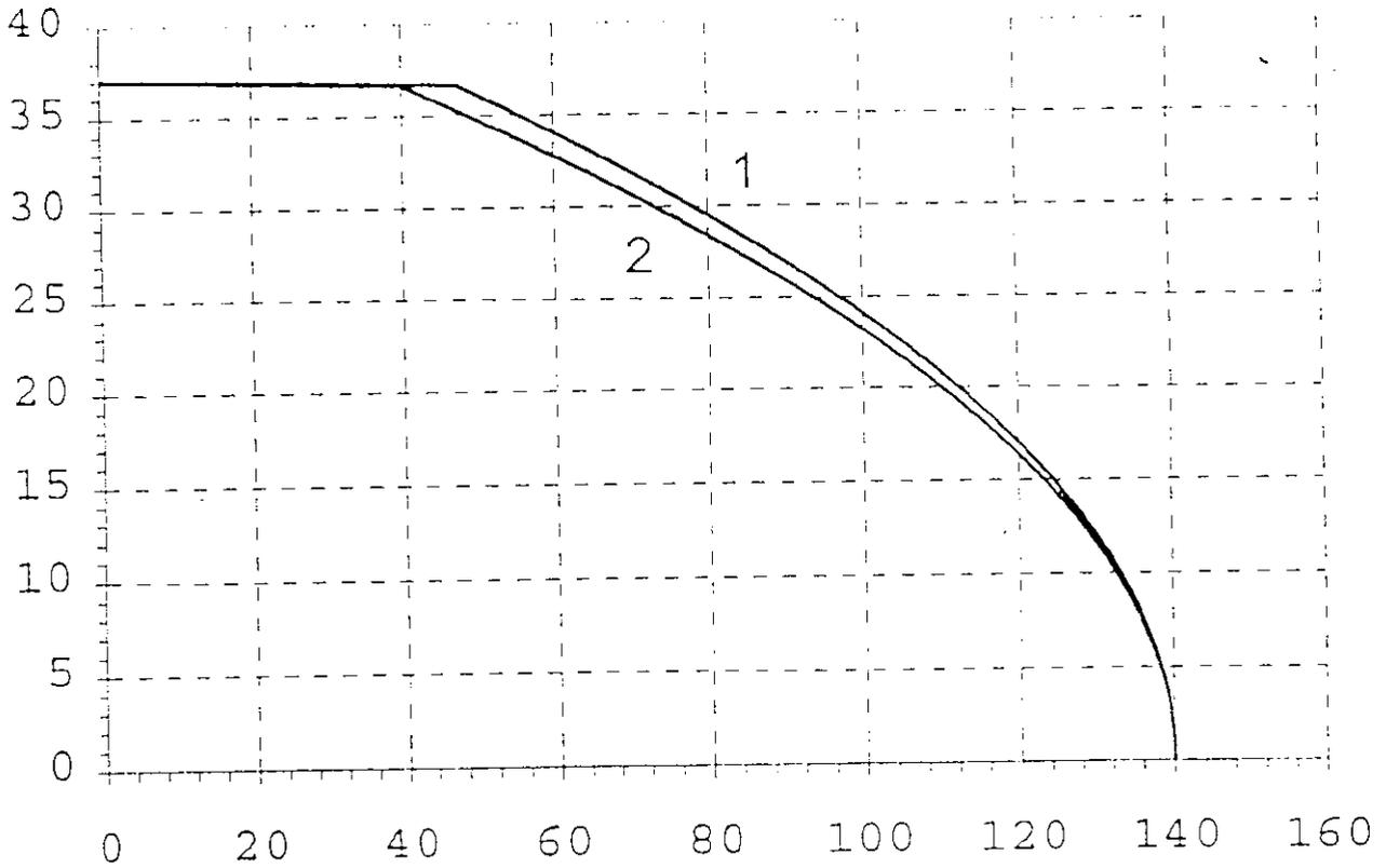
Diagram 4f : current carrying capacity (before and after electrical stress test)
