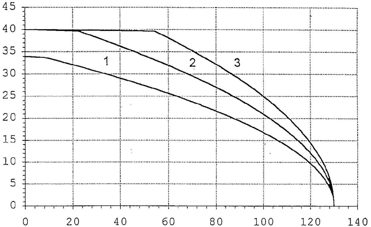
Diagram 2c : current carrying capacity „free in air“
