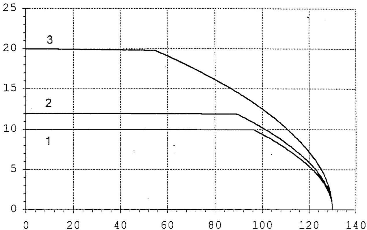
Diagram 2b : current carrying capacity „free in air“
