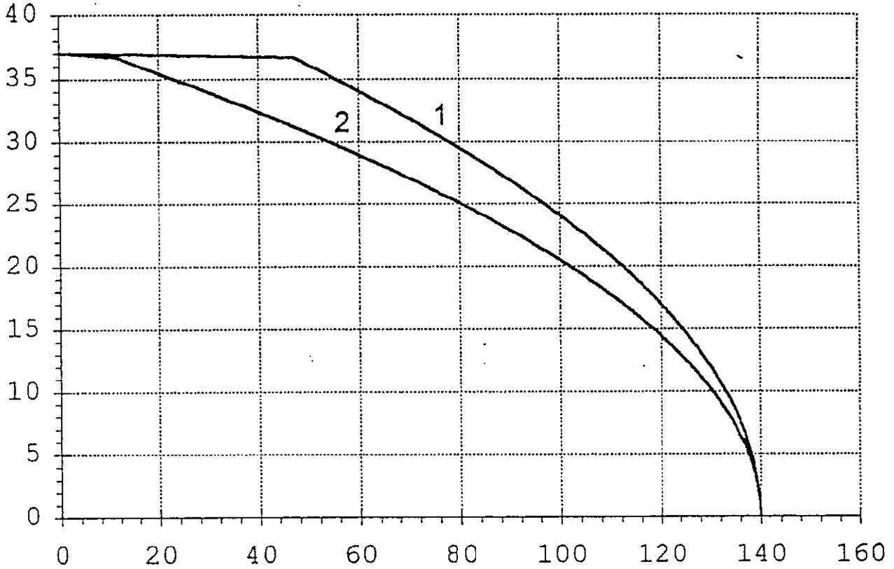
Diagram 3f : current carrying capacity in housing
