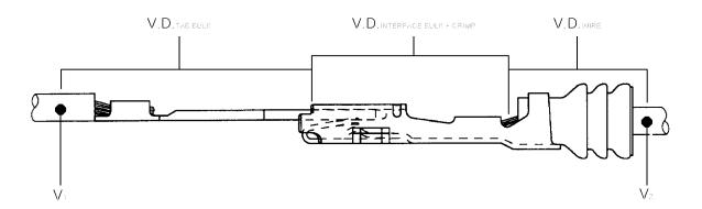
The applicable quality inspection plan shall specify the sampling acceptable quality level to be used. Dimensional and functional requirements shall be in accordance with the applicable product drawing a TOTINS SPECIFICATION (BETWEEN  $V_1 \& V_2$ ) =  $V.D._{TAB BULK} + V.D._{INTERFACE BULK CRIMP} + V.D._{WIRE}$
