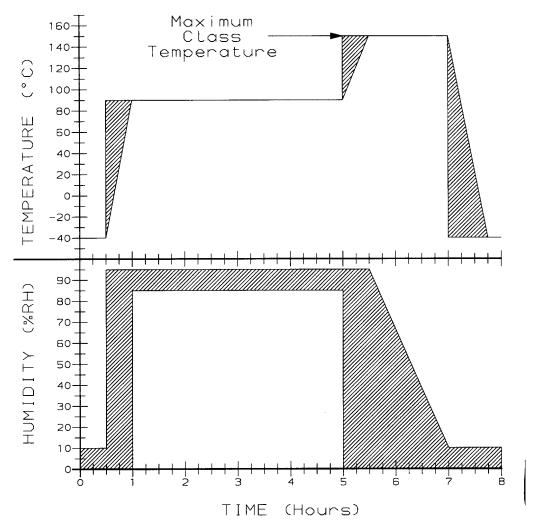
Figure 8 Humidity-Temperature Cycling Profile
