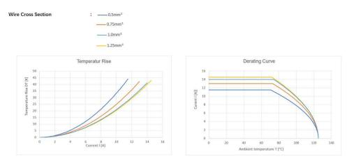
NOTE: The limit temperature as well as the maximum current carrying capacity of the used wires must be considered.
