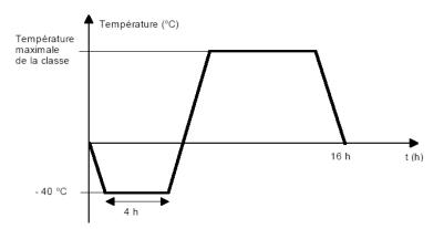
Tmin = -40°C Tmax = +100°C Temperature variation: 40°C/hour Maintaining at extreme temperature: 4h
