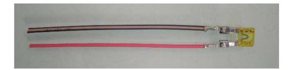
The wire length is 100mm. The resistance of: The fuse, The two wires are removed from the resistance measurement. The criterion of acceptance is the sum of both connexions on the both fuse tabs.
