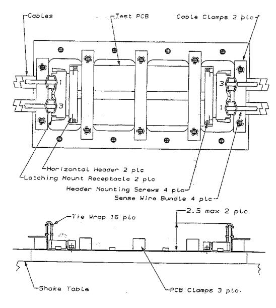
Figure 6 Vibration and Physical Shock Mounting Fixture
