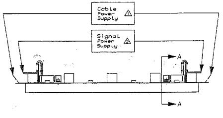
$\triangle$  Typical power supply connection for termination resistance of power contacts.  $\triangle$  Typical power supply connection for termination resistance of signal contacts.
