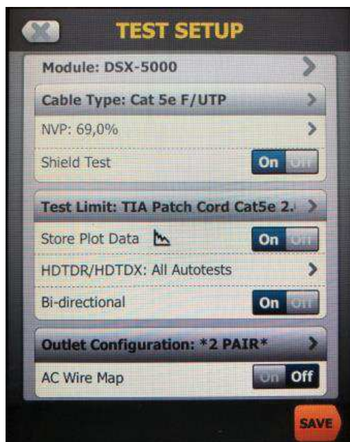
Figure 3 – Example Category 5e Test Setup
