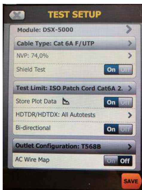
Figure 1 – Example Category 6A Test Setup
