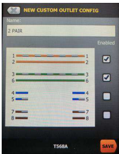
Figure 2 - Example Two-Pair Custom Outlet Configuration
