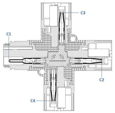
Figure 2, T- Splitter and Multi Splitter
