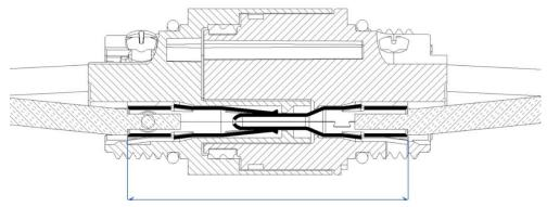
Figure 1, In-Line connector
