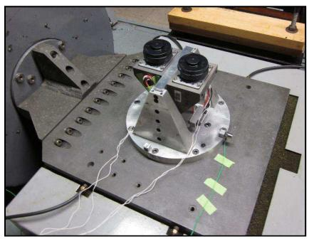
Figure 5 (Vibration and Mechanical Shock Mounting Fixture)
