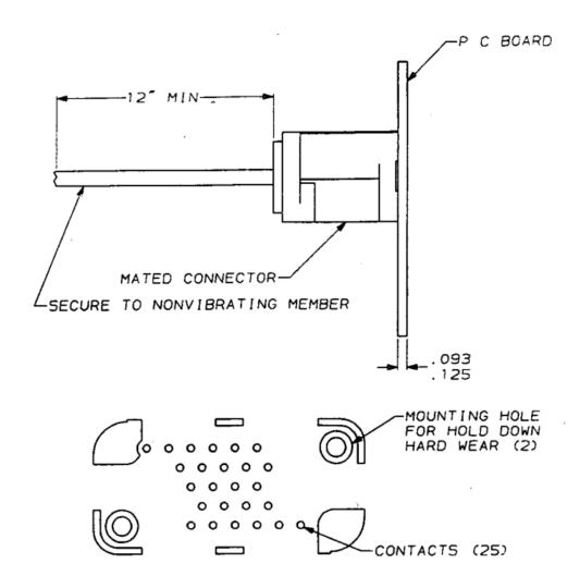
VIBRATION LEVEL IS APPLIED TO THE SPECIFIED CONNECTOR MOUNTING AREA OF THE P. C. BOARD
