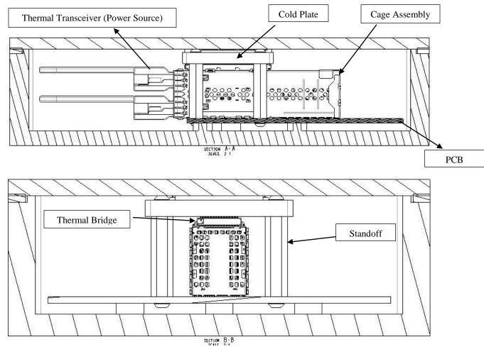
Figure 2: Section views of Thermal Bridge Thermal Measurement Test Setup
