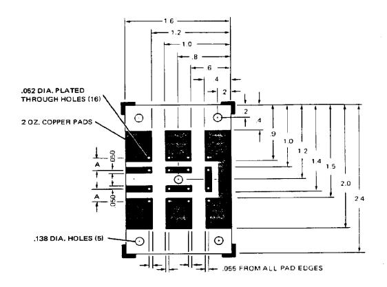
$^{\prime\prime}A^{\prime\prime}$  dimension -- .200 or .250 inch between hole centerlines, as applicable for contacts being used.
