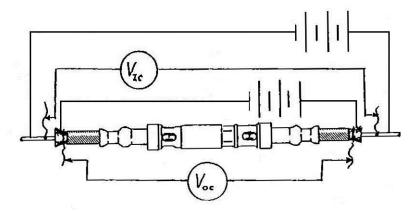
Note: a) Measure voltage drop at specified current and calculate resistance.
