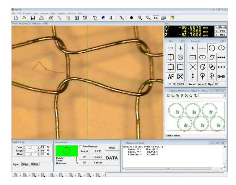
Use of the non-contact measuring machine can assist with difficult measurements and counting of the wire filament of the knitted bandage.
