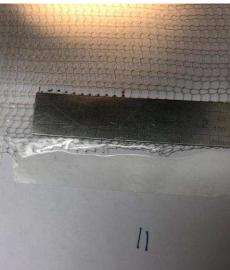
Measurement and counting of stitches along a linear inch of knitted wire mesh bandage.
