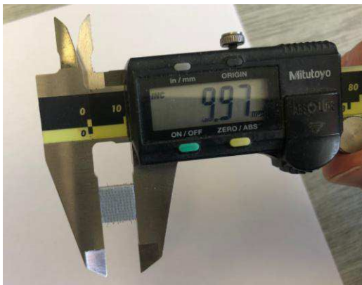
Measurement of standard samples in preparation for wire count measurement.
