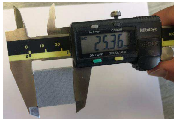
Measurement of standard samples in preparation for wire count measurement.
