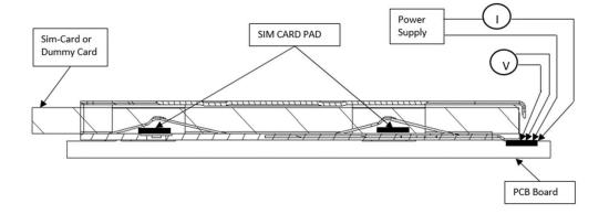
Fig.4 Termination Resistance Measuring Points
