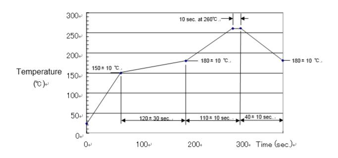
Fig.3 Reflow temperature profile
