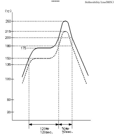
Fig. 3 Reflow Condition
