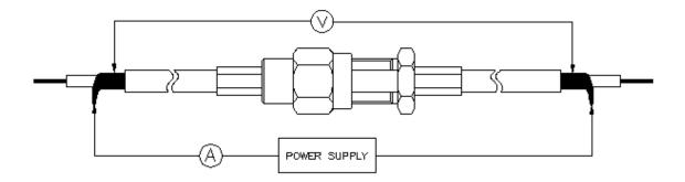
Figure 3 Typical LLCR Measurement Points
