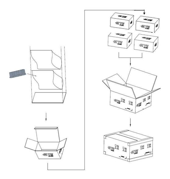
Step 1: Put the urethane foam on the bottom of inner box.
