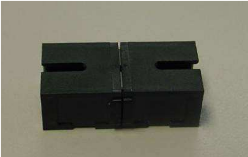
NOT ACCEPTABLE Gap Between Housings SC Figure 19
