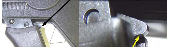
LIFT Pawl UP to "RELEASE" crimp Ratchet and OPEN Crimp Jaws
