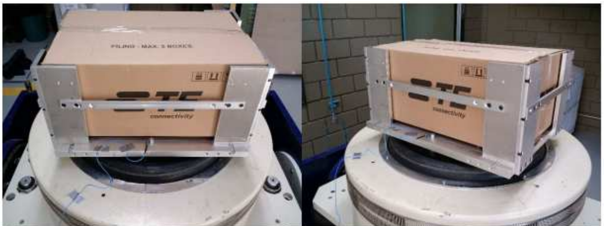
Samples inside box under shipping vibration test
