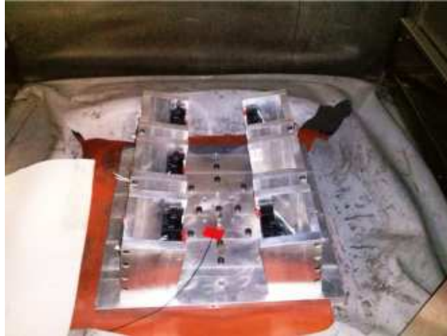
Samples under fretting corrosion test
