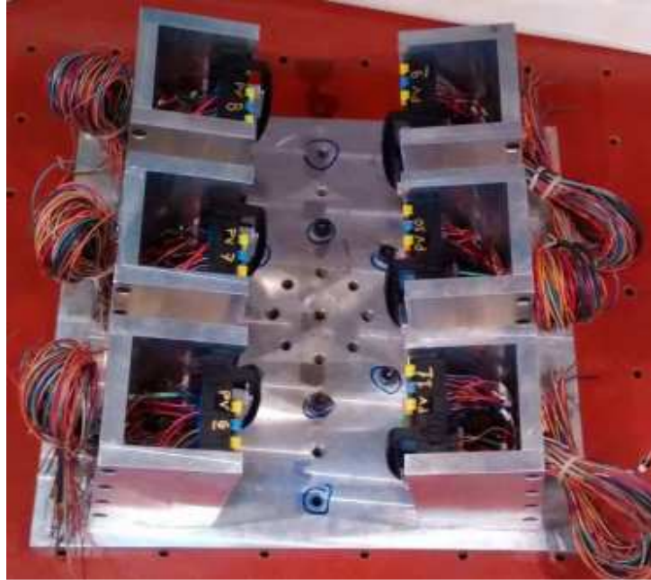
Samples mounted in the fixture for mechanical shock and vibration tests.
