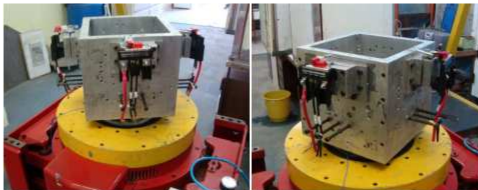
Samples under fretting corrosion test
