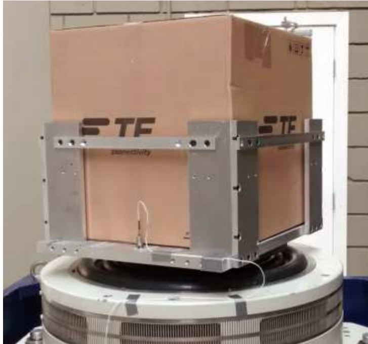
Samples inside box under shipping vibration test
