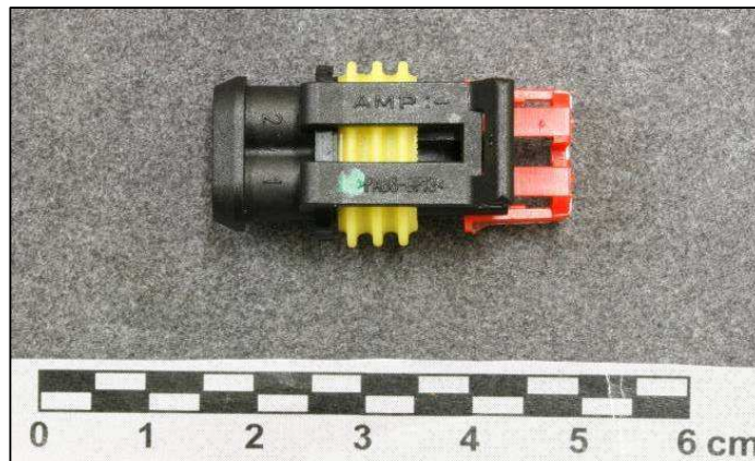
Photo 11 - AMP SUPERSEAL 1.5 SRS. 2 POSITIONS PLUG ASS'Y, PN 282080-1
