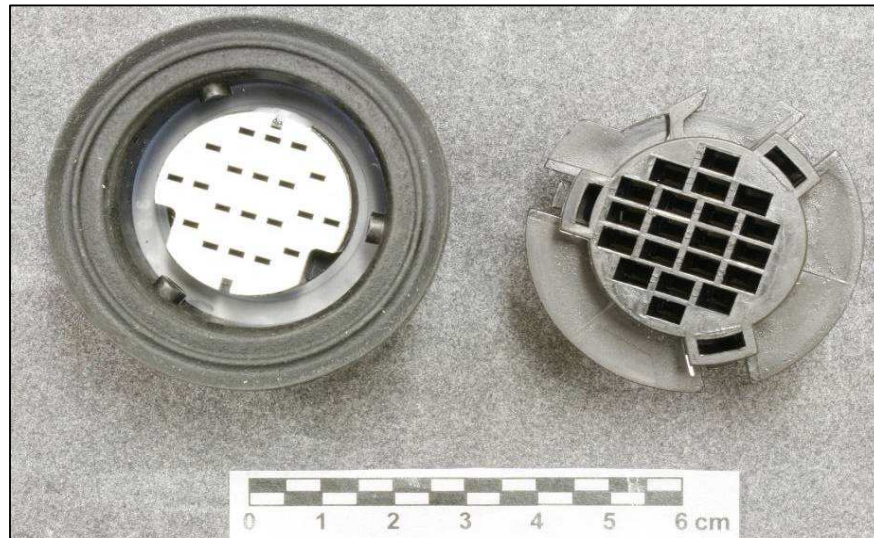
Photo 14 - HOUSING DOOR'S OFF ASSY 20POSN MULTILOCK REC PN 881637-3 AND TAB PN 881643-3, RESPECTIVELY
