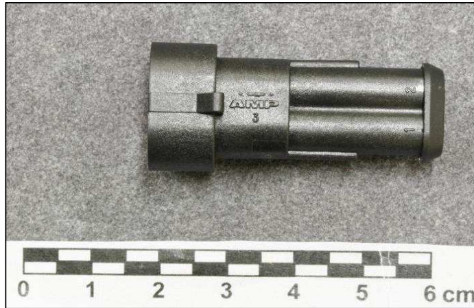
Photo 12 - AMP SUPERSEAL 1.5 SRS. 2 POSITIONS TAB ASSY, PN 282104-1
