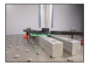
Figure 11- Typical Compliant Pin mounting force onto PCB test setup.
