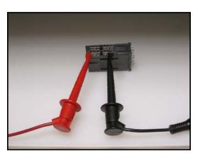
Figure 4- Front to Back Withstand Voltage test setup
