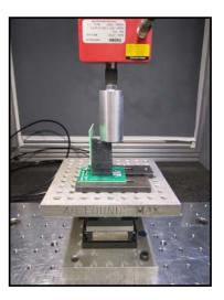
Figure 9- Mating Force Test Setup
