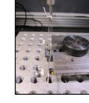
Figure 13- Terminal Retention Force, Blades
