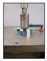
Figure 12- Typical Compliant Pin push-out force test setup.
