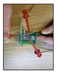
Figure 1- Low Level Contact Resistance test setup
