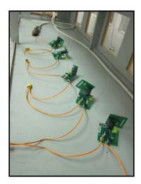
Figure 6- Temperature Rise vs. Current test setup
