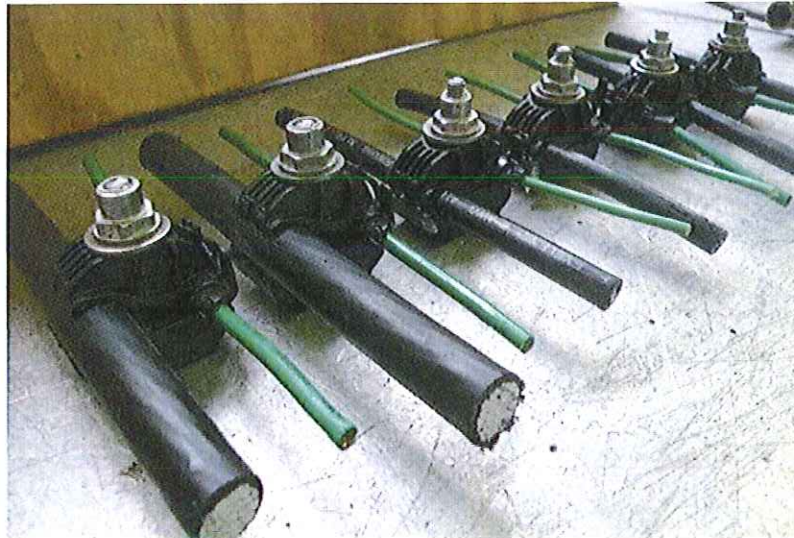
View of the connectors after been tightened at 120% of the nominal torque.
