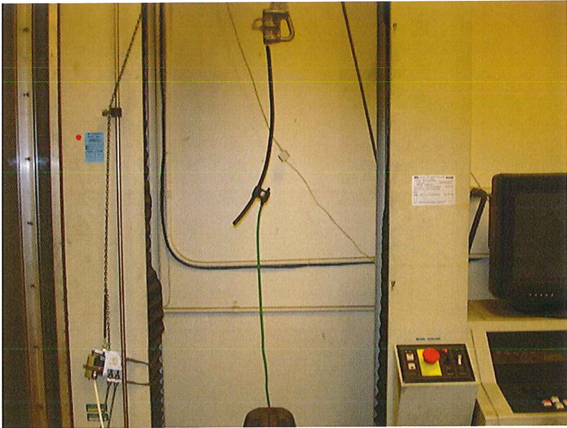
Representative photograph of KZEP 4/0 P/N 1-0708052-1 test set-up for Tensile Strength & One Minute Load tests (Group 1) ANSI C119.5-2009
