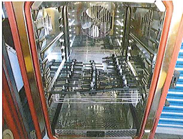
View of the connectors pre-fitted inside the hot-cold chamber.
