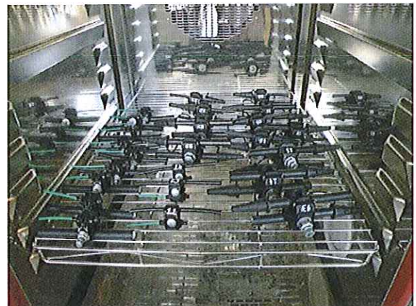
View of the connectors pre-fitted inside the hot-cold chamber.
