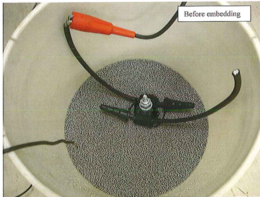
Representative photograph of KZEP 4/0 P/N 1-0708052-1 set-up prior to being embedded in 7 1/2 shot during Insulation Puncture test
