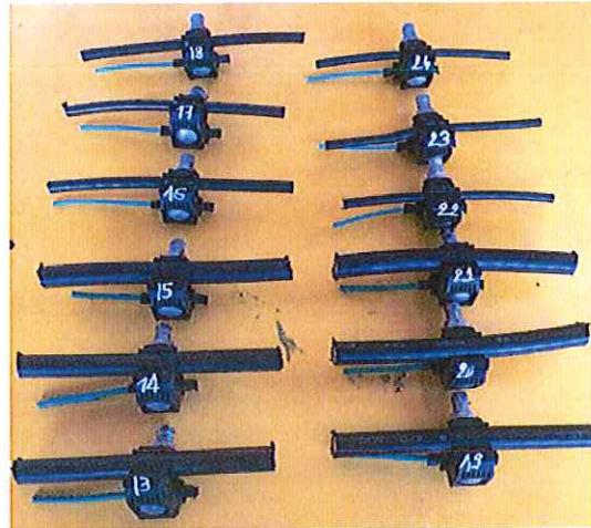
View of the connectors pre-fitted before placing in the hot-cold chamber.
