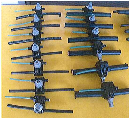
View of the connectors pre-fitted before placing in the hot-cold chamber.
